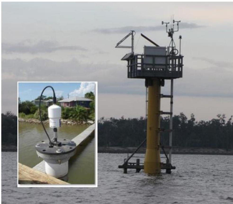
**Figure 2-2.** An elevated NOS/CO-OPS NWLON station using an Aquatrak acoustic WL sensor (inset) with a sounding tube housed inside a protective 6-inch PVC well. Photo courtesy of NOS/CO-OPS.
