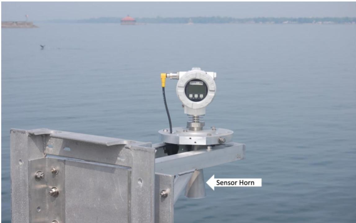
**Figure 2-1.** Xylem/Design Analysis H3611 microwave water level sensor as installed by NOS/CO-OPS. Photo courtesy of NOS/CO-OPS.
