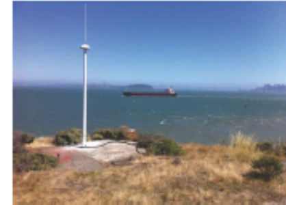
Figure 1. IOOS operates the nation's only network of land-based high-frequency radars (pictured above) that provide continuous, real-time mapping of the speed and direction of surface currents in coastal waters.
