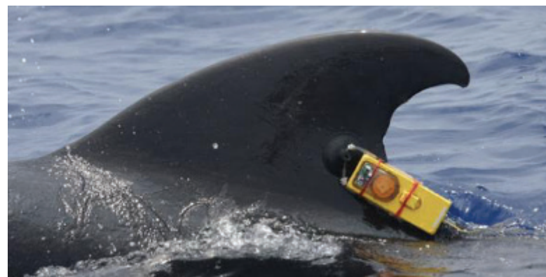
A Wildlife Computers Mk10-F satellite tag joined with a Telonics VHF transmitter and Fastloc GPS, mounted on a short-finned pilot whale in Hawai'i. Photo Credit: Greg Schorr and Robin Baird—NMFS Permit # 731-1744 issued to Robin Baird
