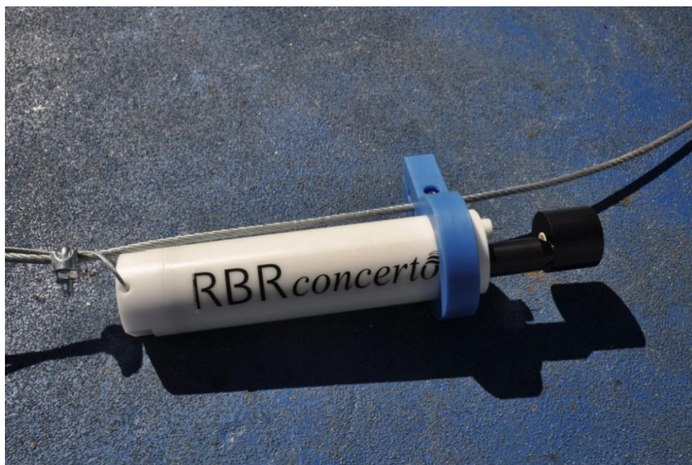
Figure 2-3. This towed RBR concerto CTD uses an inductive conductivity sensor with an external field and no pump (photo courtesy of Igor Shkvorets/RBR Ltd.).
