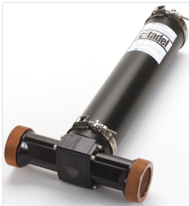
Figure 2-5. The Teledyne RD Instruments Citadel CTD-NH (discontinued in 2019) is an example of an inductive sensor with a constrained field (photo courtesy of Paul Devine/Teledyne RD Instruments).
