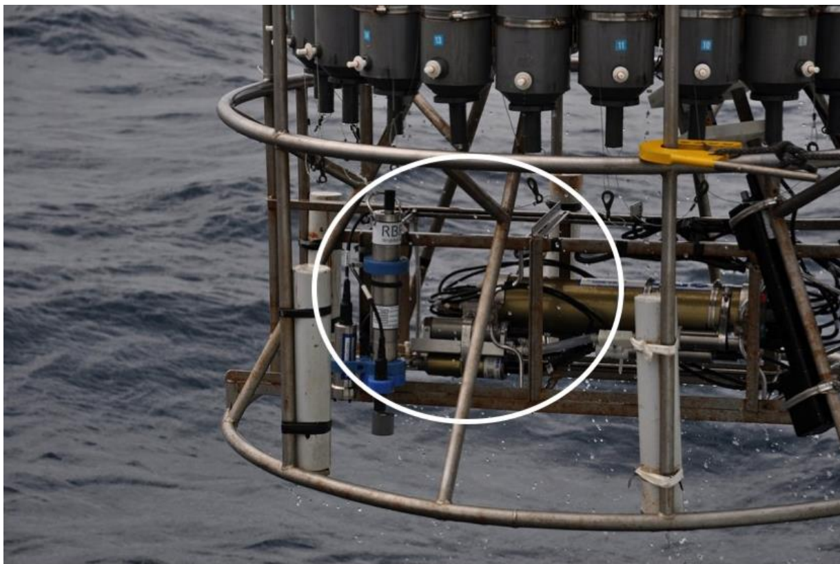
Figure 2-9. This CTD/bottle rosette shows the use of both Sea-Bird Scientific (SBE 9plus) and RBR sensors (photo courtesy of Igor Shkvorets/RBR Ltd.).
