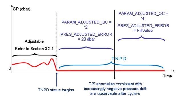
All TNPD data should receive a standard label in SCIENTIFIC\_CALIB\_COMMENT in the Argo single-cycle netcdf files, in the dimension corresponding to PRES. The standard label consists of the character string "TNPD: APEX float that truncated negative pressure drift". The delayed-mode operator may append to the end of this character string any other comments regarding PRES that he/she wishes to make.
