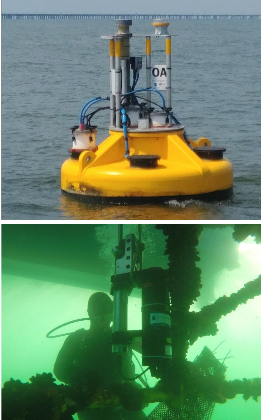
Figure 2-1. (Top) This Pacific Marine Environmental Laboratory buoy was deployed in April 2018 in the mouth of the Chesapeake Bay, where acidification may be more rapid due to a reduced buffering capacity in comparison to the open ocean (photo courtesy of M. Bushnell). (Bottom) A Sea-Bird Scientific Deep SeapHOx V2 deployed on a fixed mooring at Washington State's Carr Inlet by Northwest Environmental Mooring Group (photo courtesy of Sea-Bird Scientific and University of Washington Applied Physics Laboratory).
