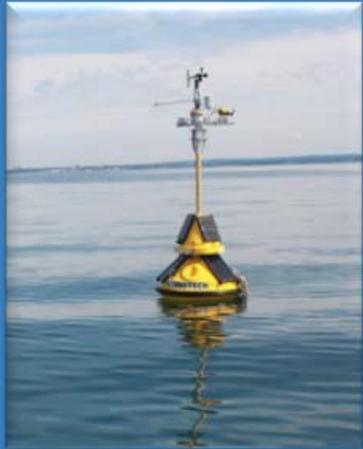
Great Lakes Observing System Hypoxia Warning System buoy deployed north of Cleveland, Ohio. These observations support water managers. Photo credit: Ed Verhamme, LimnoTech
