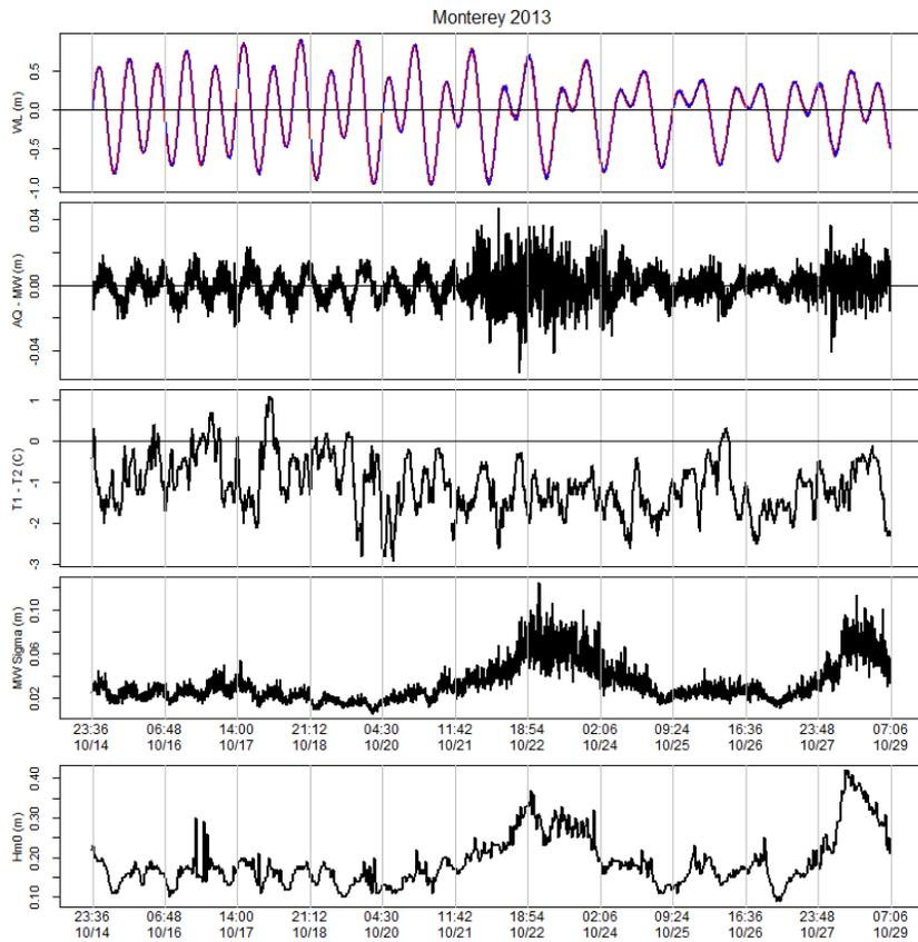
Figure 42. Monterey data for October 14 - 29, 2013. WL is the demeaned DQAP water level, microwave data are red, acoustic data are blue. AQ - MW is the water level difference. T1 - T2 is the temperature difference of the two thermistors. MW Sigma is the DQAP standard deviation ( $\sigma$ ) of the microwave data.  $H_{m0}$  is the significant wave height.
