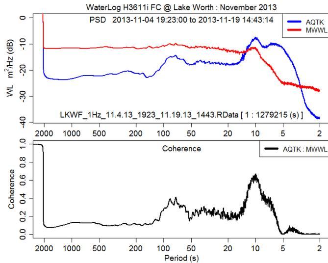
Figure 36. PSD and coherence of acoustic and microwave water level data at Lake Worth for November 2013.
