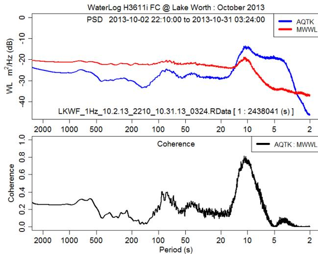
Figure 34. PSD and coherence of acoustic and microwave water level data at Lake Worth for October 2013.
