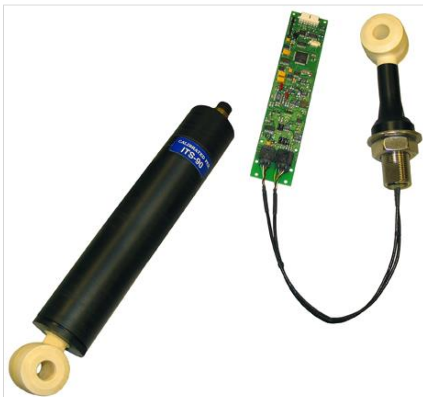
Figure 2-4. The Teledyne RD Instruments CITADEL CTD-ES is an example of an inductive sensor with an external field. Operators must be certain that additional hardware is sufficiently distant from the toroid to avoid interference. This sensor is designed for simple and easy cleaning (photo courtesy of Paul Devine/Teledyne RD Instruments).
