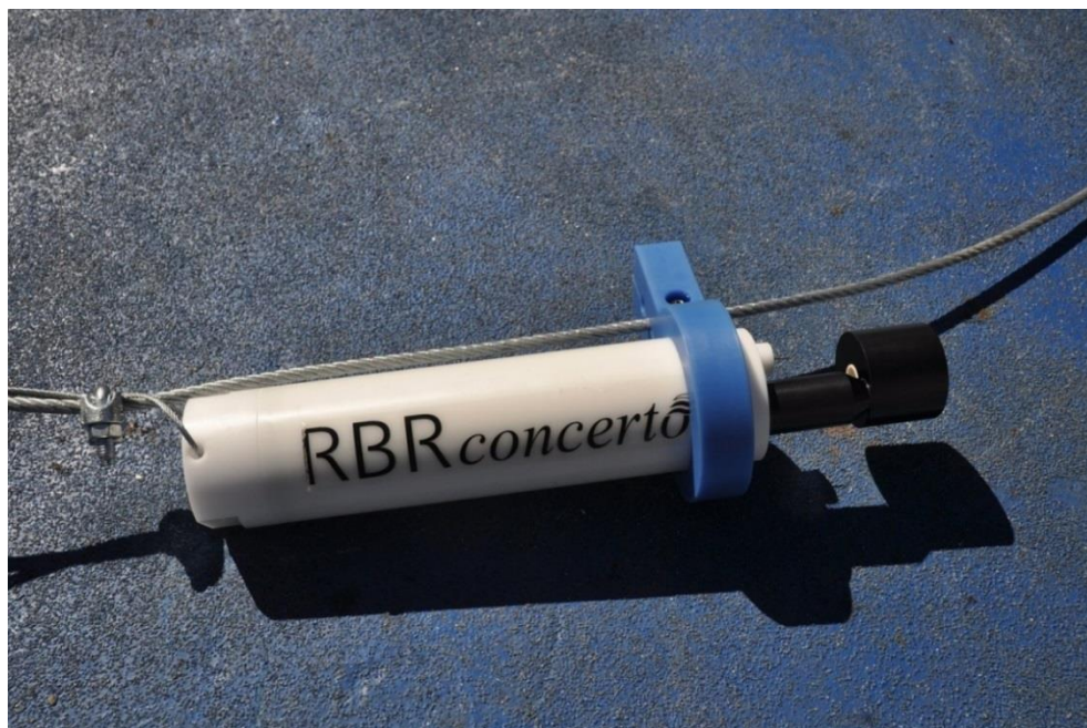
Figure 2-3. This towed RBR concerto CTD uses an inductive sensor with an external field and no pump (photo courtesy of Igor Shkvorets/RBR Ltd.).
