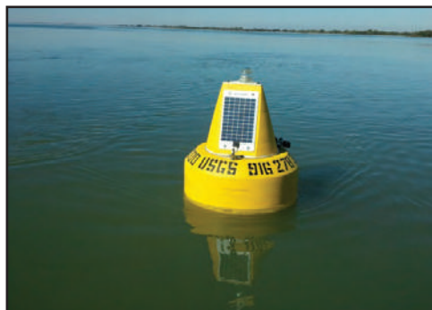
Figure 13. Ultraviolet (UV) nitrate sensor deployment infrastructure showing A , pipes; B , instrument cages; C , pumped applications (gage house); and D , buoy deployments. Photos courtesy of Jessica Garrett, U.S. Geological Survey; Jacob Gibs, U.S. Geological Survey; JohnFranco Saraceno, U.S. Geological Survey; Bryan Downing, U.S. Geological Survey.
