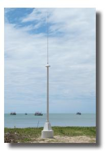
Photo 3: Present-day Coastal Ocean Dynamics Applications Radar (CODAR) having combined transmit and receive antennas in one unit. (Total height is approximately 8 meters for this particular unit).
