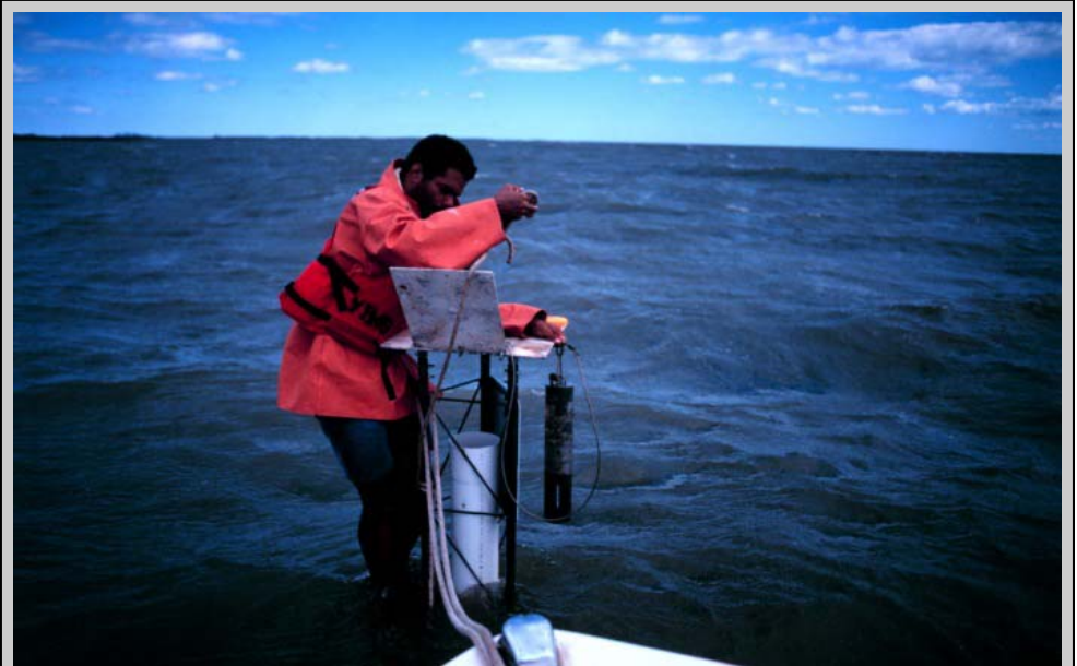
Water quality sampling taking place on an offshore data-logger station in a protected area. Photo: April Bahen, CBNERRVA
