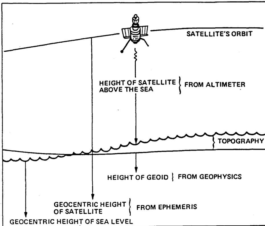
Figure 1: The basic geometry of satellite altimetry (from Stewart and al, 1983).
