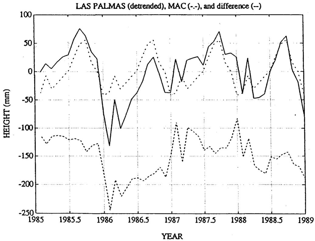
Figure 12b. Monthly data with trend removed (solid line) superimposed with the Mean Annual Cycle (MAC) above and detrended monthly data minus the MAC (below). With the trend removed, the data appear reasonable.
