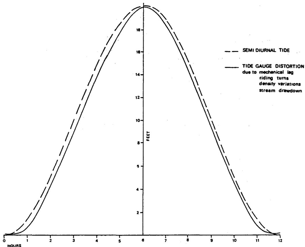
Comparison between the hypothetical open water tide and the curve produced by a gauge.
