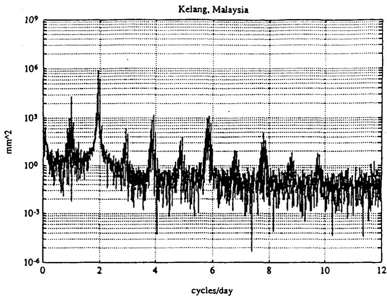
Figure 9a. Tidal spectrum with significant shallow water components.
