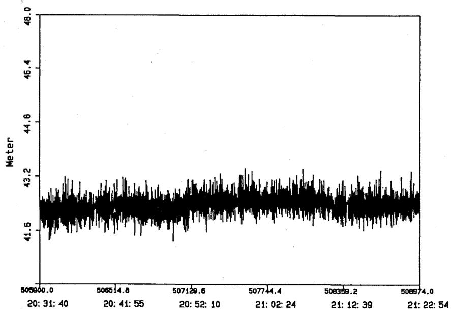
GPS AND RADAR ALTIMETER COMPARISON
