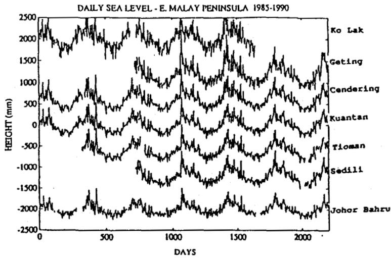
Figure 10. For regional stations, overlays of daily data plots are useful for examination of the stability of the reference level. In this case, the sea level is highly coherent and no obvious reference level shifts are present.
