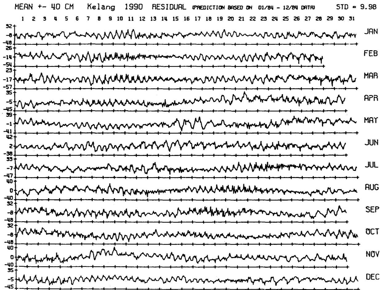
Figure 9b. Hourly residuals displaying shallow water, non-linear fluctuations due to the inability of the tidal analysis to resolve these higher frequency tidal components. These high-quality data are from a digital float and well gauge that samples every 10-seconds with 50-second averages, which in turn are decimated to hourly with a five-point filter.
