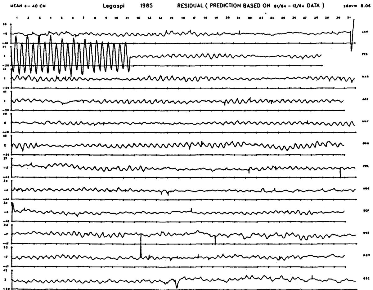
Figure 8b. Residuals of the hourly data showing a timing offset of exactly one hour in early February and many data spikes. The data are from an A.OTT float and well analog gauge that have been spot sampled on the hour. The timing shift and spikes were correctable.
