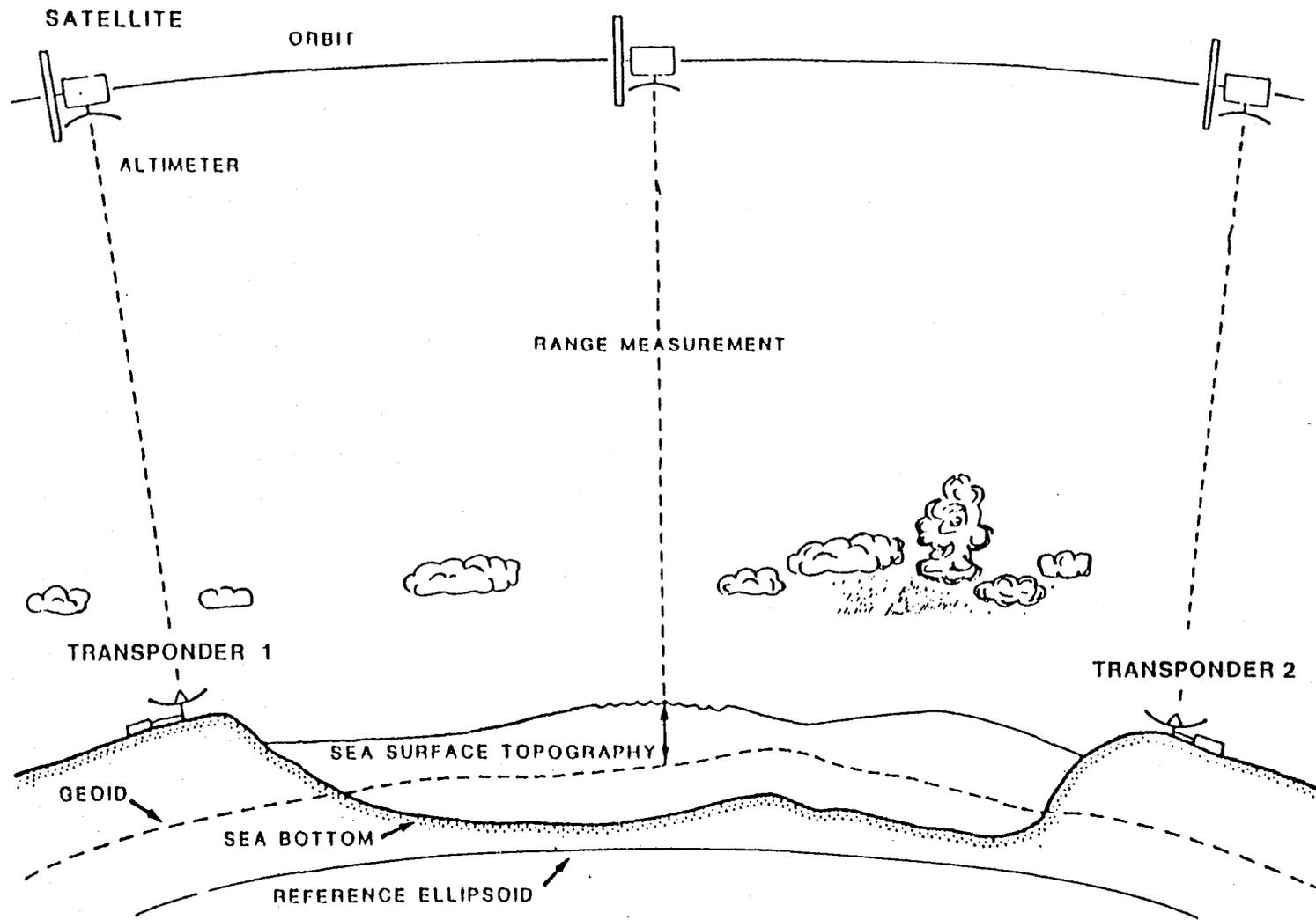
**Fig. 3** The location of transponders beneath orbit arcs crossing major oceans can potentially provide very precise mid-ocean measurements of sea surface related to positions on land.
