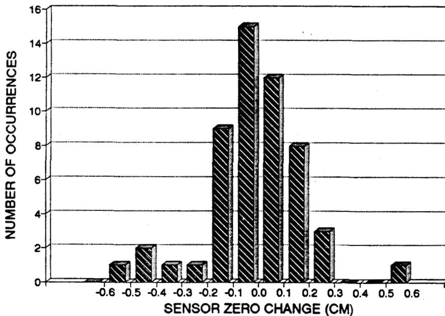
**Figure 1.** (a) Results from the post-deployment calibration check for 53 NGWLMS acoustic sensors; (b) the change in the sensor zero offset based on the post-calibration checks (the sensor zero offset is used to directly relate the sensor measurements to the local benchmarks). In both plots x-axis values are the boundary values for the interval represented by each bar.
