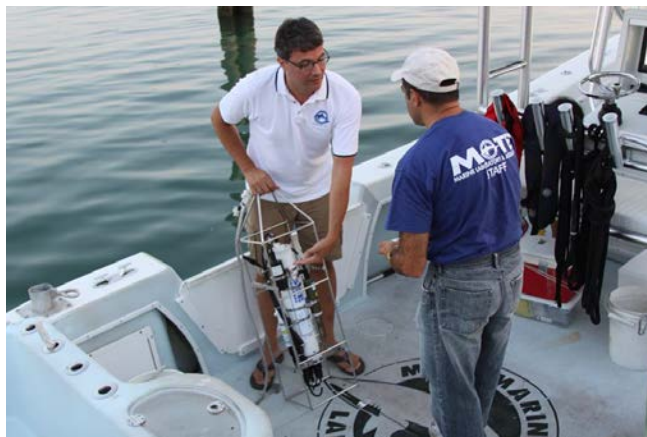
Figure 10. Researchers preparing to deploy a CTD meter to obtain environmental parameters during a Karenia brevis bloom.
