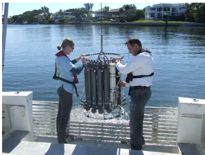
Figure 9. Researchers preparing to deploy a rosette with a CTD meter and sampling bottles.
