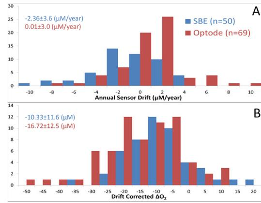
**Figure 2.** Histogram of sensor drift (A) and the Drift Corrected Average Deep  $\Delta O_2$  (B) for the two different types of oxygen sensors. The mean±std. dev. is labeled on the plot with its corresponding color.
