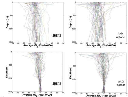
**Figure 4.** Compiled uncorrected (top) and corrected (bottom) depth profiles of the average  $\Delta O_2$  for SBE43 (n = 50) and Optode (n = 69); each line represents averages of all profiles available for a single profiling float.
