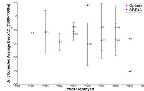
**Figure 3.** Drift Corrected Average Deep  $\Delta O_2$  as a function of deployment date. The dots represent the mean, and the error bars are  $\pm 1SD$ .
