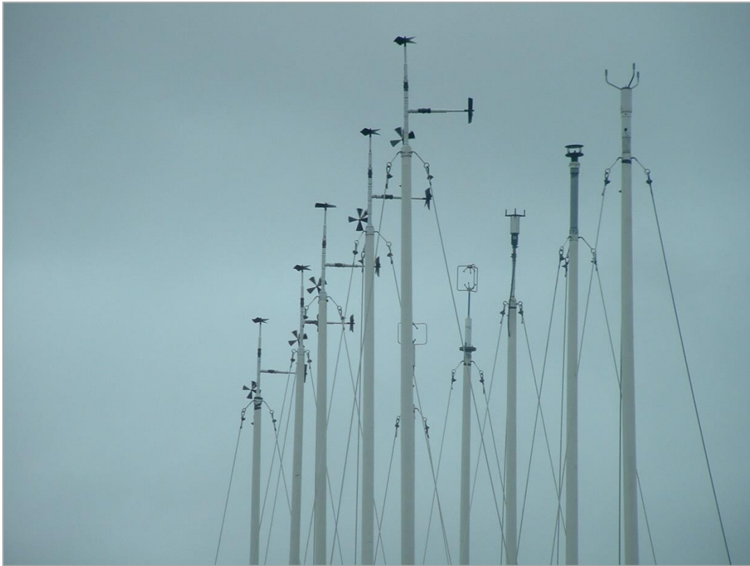
Figure 2-4. Acoustic anemometers at the Otis Weather Test facility in Cape Cod, Massachusetts. The five masts on the left provide reference wind observations. The five sensors on the right are: 1) RM Young 3-axis ultrasonic anemometer (partially obscured), 2) Gill R3 3-D anemometer, 3) RM Young 2-axis ultrasonic anemometer, 4) Gill Windsonic 2-axis ultrasonic anemometer, and 5) Vaisala WS425 ultrasonic anemometer (photo courtesy of Mark Bushnell).
