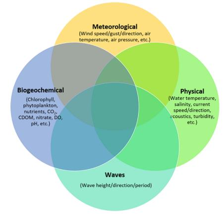
*Figure 5.* Groupings of variables observed on coastal moorings. Moorings can host numerous sensors, and most moorings observe multiple variables. One mooring can fall into several observation categories.
