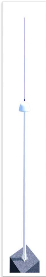
Figure E-2: A CODAR SeaSonde Antenna
