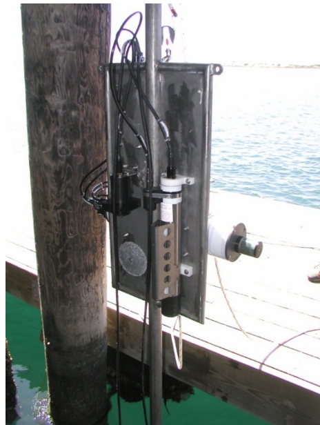
Figure D-15: National Estuarine Research Reserve (NERRS) water quality station
