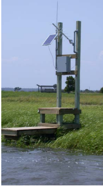
Figure D-15: National Estuarine Research Reserve (NERRS) water quality station
