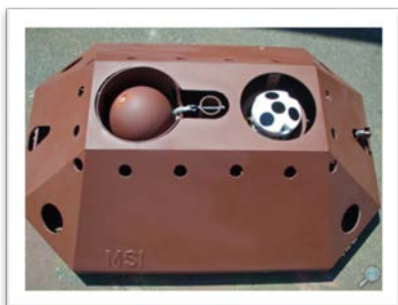
Figure D-3: Mooring Systems, Inc., Miniaturized Trawl Resistant Bottom Mount (MTRBM)
