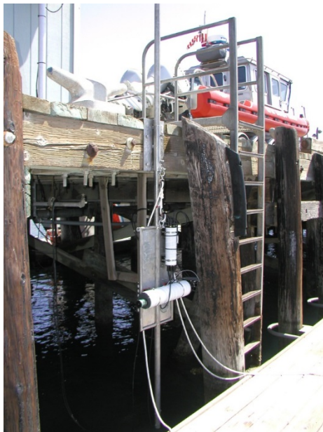
Figure D-15: National Estuarine Research Reserve (NERRS) water quality station
