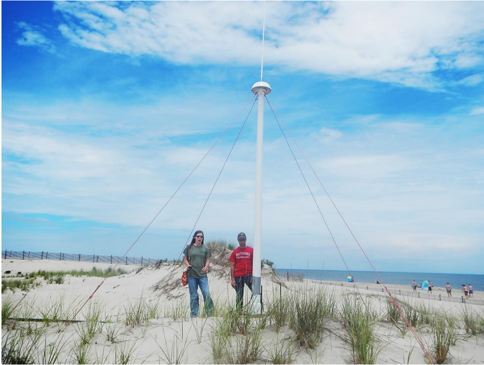
Figure 3-1. A 25 MHz combined transmitting and receiving antenna deployed at Cape Henlopen, Delaware.
