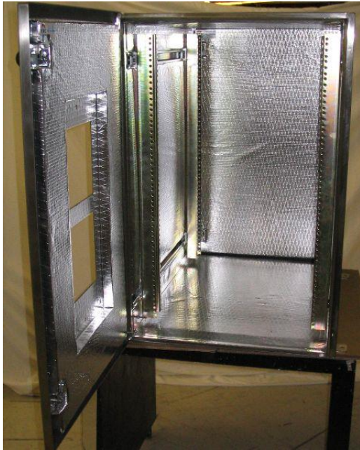
Figure 1. Interior of empty outdoor electronics enclosure without air-conditioner attached.
