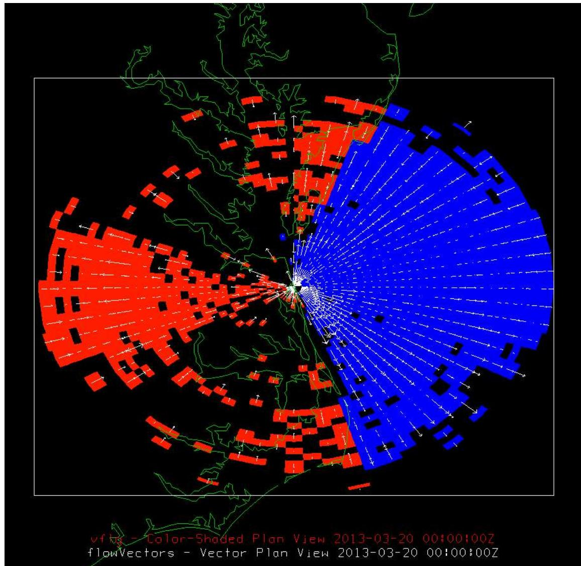
Figure 1. CODAR radial velocities plotted over vector flag values. Red vector flags represent solutions outside the valid sample domain.
