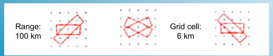
Integration areas for a pair of 16 antenna WERA systems at about 100 km distance from the radar.
