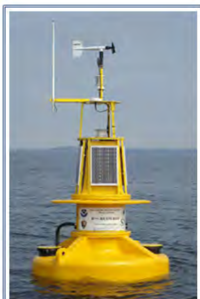
Water quality data are collected from sensors attached to a Chesapeake Bay Interpretive Buoy System (CBIBS) buoy.
