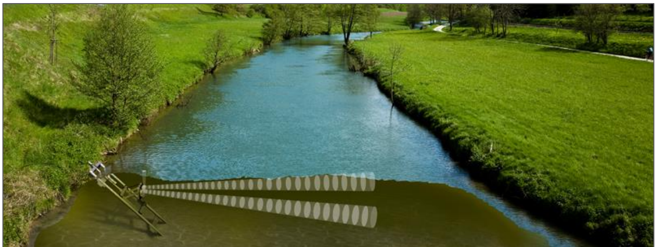
Figure 2-3. This illustration shows a possible deployment of a side-looking ADCP on a slanted rail system. Photo credit: SonTek.
