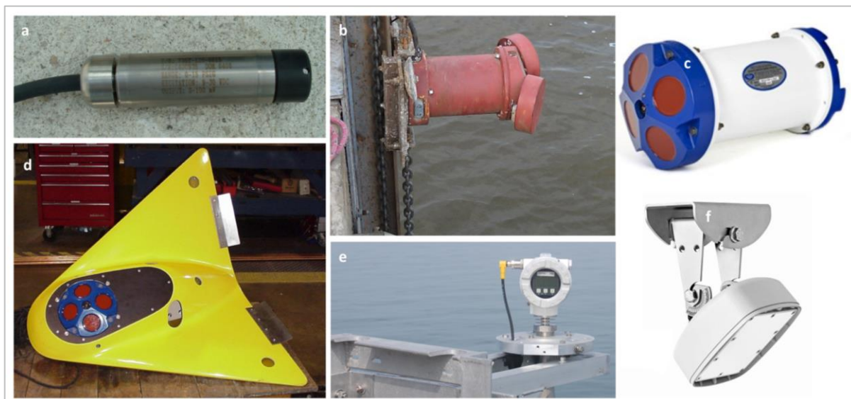
Figure 2-4. A small sample of devices used to collect data for stream flow determinations: a) KPI pressure sensor, b) SonTek SL ADP c) RDI ADCP, d) RDI ADCP in YSI fin, e) details, f) Xylem Design Analysis H3611. Photo credits: M. Bushnell, TRDI, Xylem.
