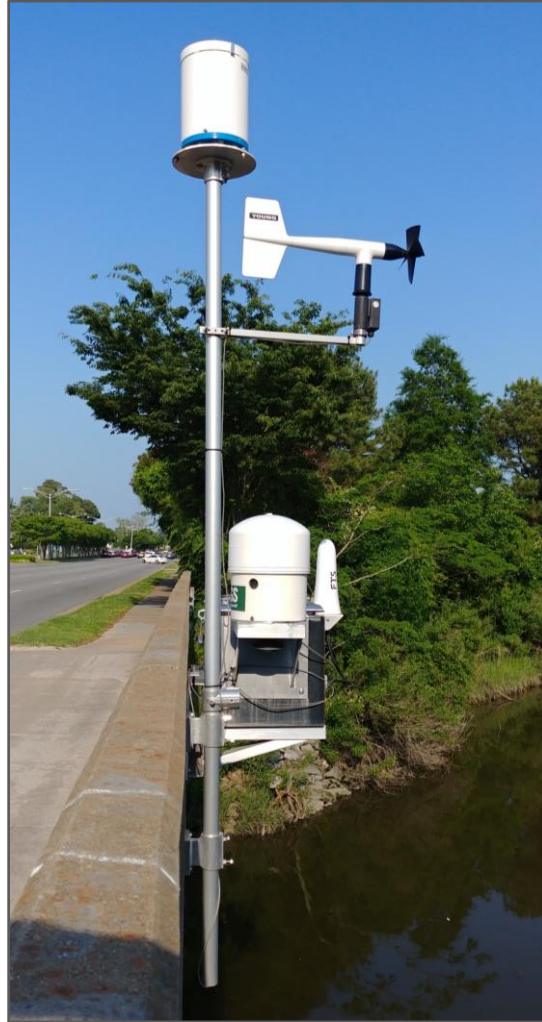
Figure 2-2. This USGS gauge is mounted on a fixed bridge and utilizes a microwave altimeter to measure water levels. The station also includes wind speed and direction, air temperature, barometric pressure, and rainfall sensors. Photo credit: M. Bushnell.
