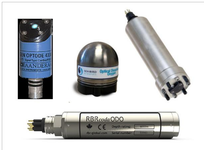
Figure 2-1. Commonly used DO sensors: Clockwise from upper left: an Aanderaa 4330 sensor, a Sea-Bird Scientific SBE 63 sensor, a JFE Advantech Rinko III Fast DO sensor, and an RBR coda ODO sensor. (Photos courtesy of Aanderaa, Payal Parikh/Sea-Bird Scientific, JFE Advantech, and RBR).
